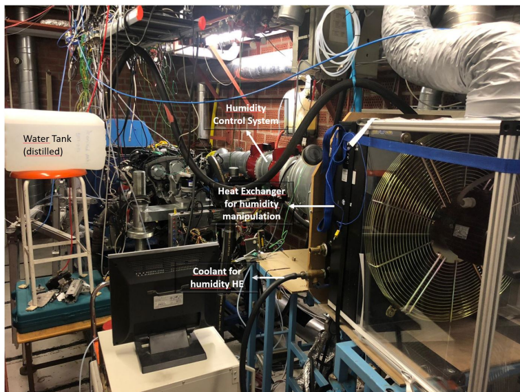
Figure 2.2: The experimental setup in the test cell comprising the GEP3 Engine and the water injection system
