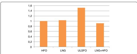
**Fig. 11** OPEX differences with different fuels and alternatives (LNG = using LNG all the time whilst LNG + HFO = HFO is used outside ECAs). Relative differences: 1 = costs running on HFO
