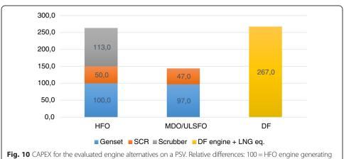
Fig. 10 CAPEX for the evaluated engine alternatives on a PSV. Relative differences: 100 = HFO engine generating set (Genset)
