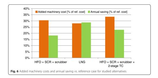
payback times by 23...28 %. Increasing only the LNG price to a ratio of 1.29\*HFO, instead of the assumed 1.1\*HFO price, will also increase the LNG case payback time to the same level as for the HFO + SCR + scrubber case and especially eventual drops in the price of MGO vs. HFO will have large implications as seen in Table 3.
