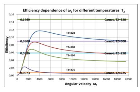
Fig 5: Efficiency dependence of  $\omega_1$  for different temperatures  $T_2$ , comparison with Carnot's limit Input data for the calculation: Ra= 0,5m; H= 0,4m; D= 0,015m; Kappa= 1,84E-09
