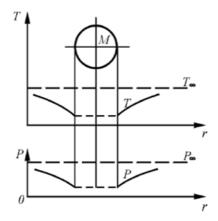
Fig. 5.17. Distribution of temperature and pressure around a conglomerate of toroidal vortexes in free space
