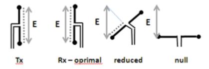
Figure 1, Comparison of conventional dipole transceiver antennas positioning.
