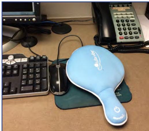
Figure 1. The vibrating device, which is placed next to the mouse to prevent the computer from automatically logging off owing to inactivity.
