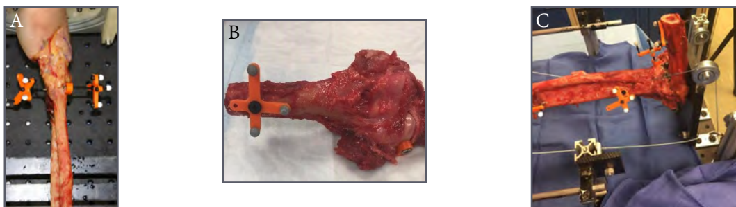
Figure 7. Various images of the forearm, showing positioning of the retroreflective markers on the 3D printed rigid bodies. (A) Distal radius and ulna. (B) Fixed humerus. (C) Proximal radius and ulna.
