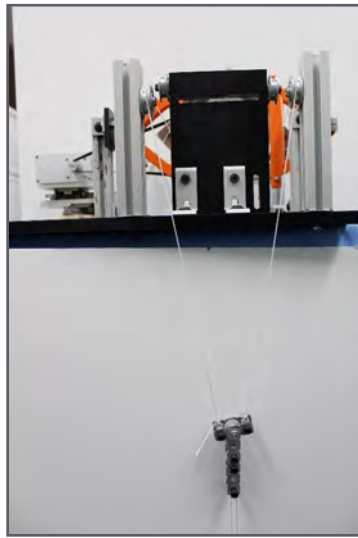
Figure 5. Pulley system showing cables routed through Y-weight distributor for axial loading of the forearm.
