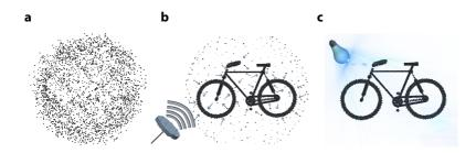
Figure 5.6: General scheme of acoustic fabrication. (a) A homogeneous dispersion is exposed to a structured ultrasound field (b), which defines trapping regions for particles. (c) UV light triggers the fixing reaction and thus permanently fixes the particles to create the object. Figure taken from reference [16].
