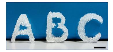
Figure 5.9: Photograph of mechanically stable and self-supporting objects in the form of letters A, B and C. Scale bar 10 mm. Figure taken from reference [16].
