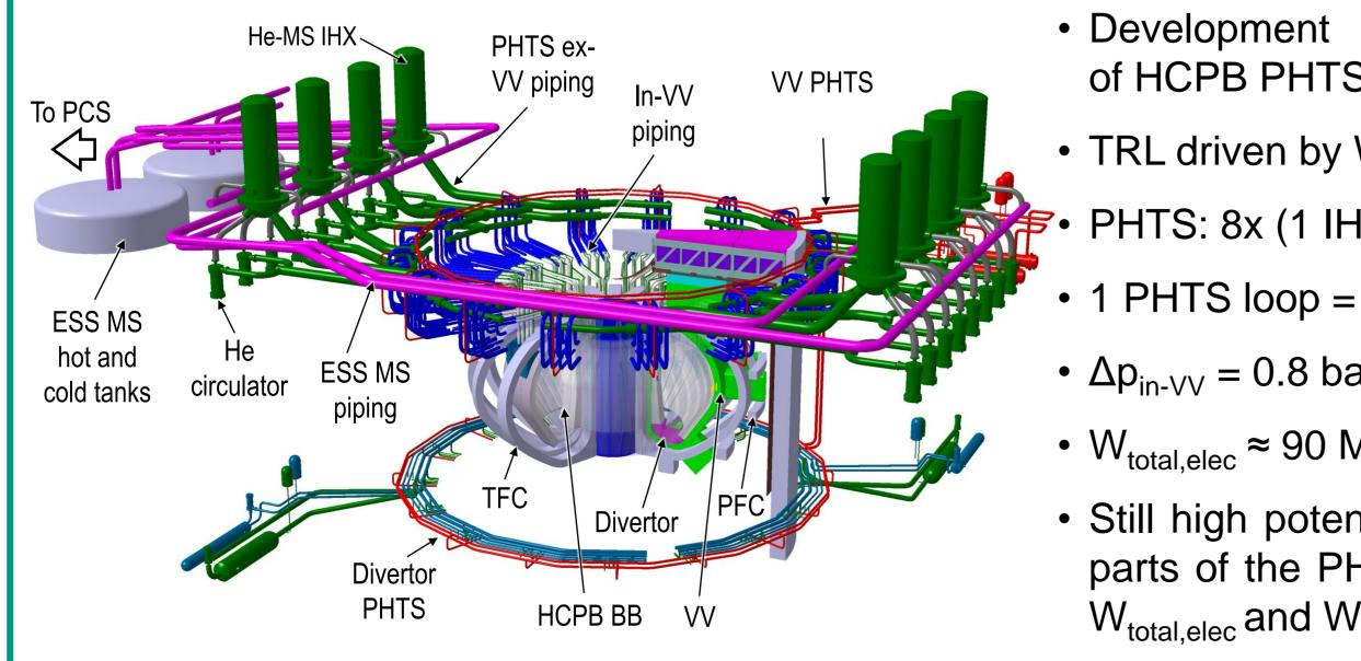
• Development target: maximization of HCPB PHTS and BoP TRL • TRL driven by W<sub>circ,elec</sub> (< 6 MW) PHTS: 8x (1 IHX + 2 circulators) • 1 PHTS loop = 2 sectors, OB + IB •  $\Delta p_{in-VV} = 0.8$  bar,  $\Delta p_{ex-VV} = 1.9$  bar • W<sub>total.elec</sub> ≈ 90 MW, W<sub>circ.elec</sub> ≈ 5 MW
