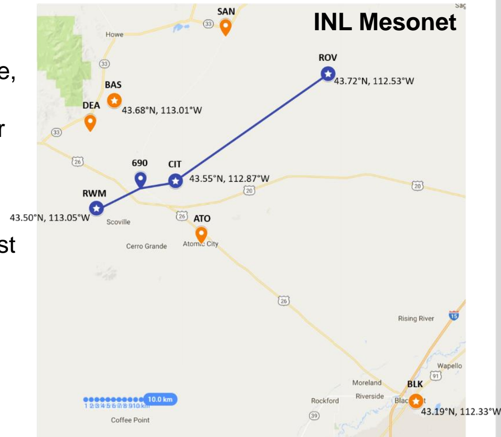
Simulated overhead line, going along weather stations from the meteorological monitoring network from the Idaho National Laboratory (USA)
