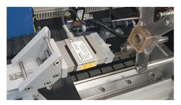
Figure 4.6: Test setup for measuring the metal membrane's force-displacement characteristics.
