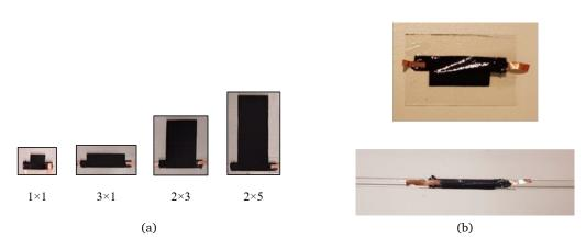
**Figure 4.25:** DES with different geometries (a), cut from the metal frame and mounted onto the polymer tube (b).
