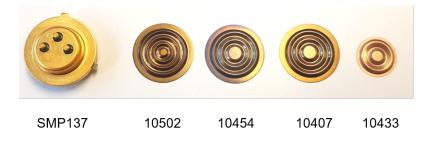
Figure 4.5: Different metal membranes in comparison to the Bosch SMP137 pressure sensor.
