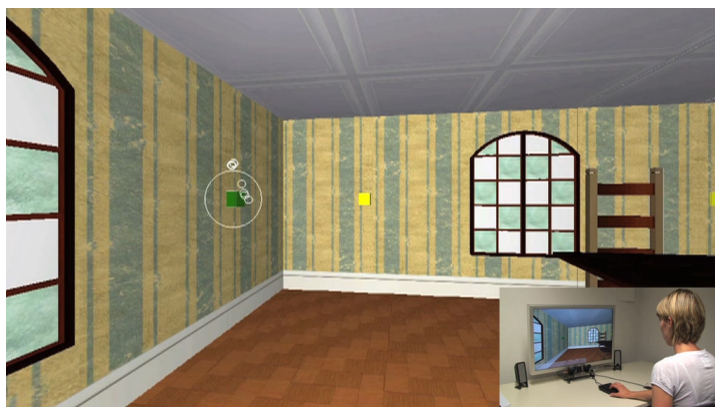
Figure 5.2: Recording user data with an eye-tracker. The image shows the eye-tracker equipment on the bottom right, the player's point of view, and circles (not shown to the player) indicating the recorded user's gaze on the current scene.
