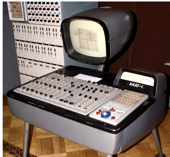
Figure 1. Modern simulations evolved from early post World War II computer simulators, such as the digital AKAT-1 used for thermodynamic simulations ( https://commons.wikimedia.org/wiki/File:AKAT-1.JPG (CC BY-SA 3.0))
