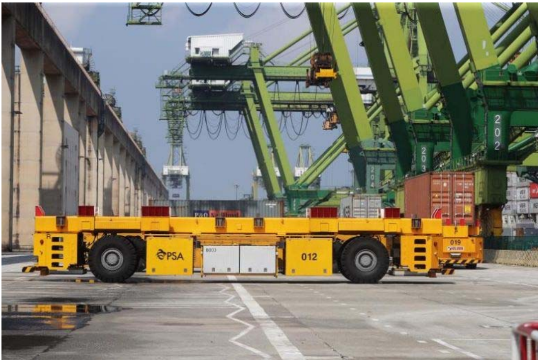
Figure 8. Driverless container carrying vehicle in Pasir Panjang terminal, Port of Singapore. Retrieved from https://www.straitstimes.com/singapore/new-automated-cranes-on-trial-at-pasir-panjang-terminal-in-boost-for-singapores-port-hub
