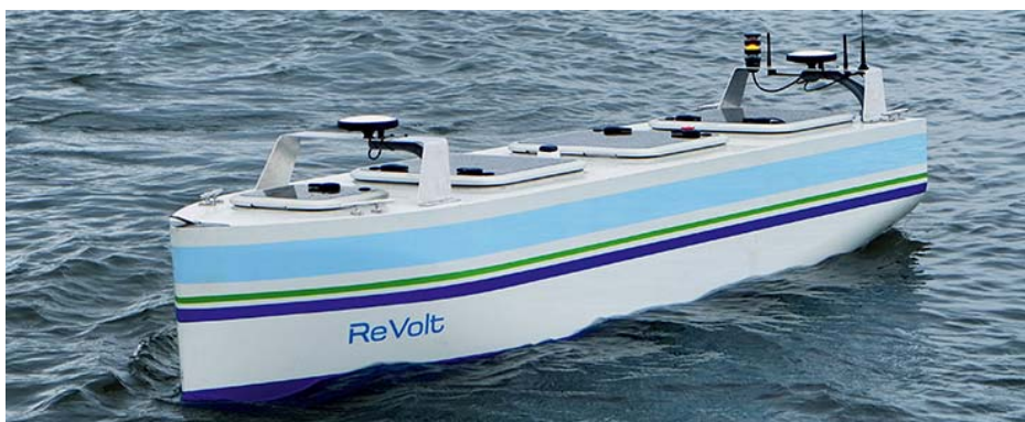
Figure 5. Downscaled prototype of The ReVolt autonomous vessel. Retrieved from: https://www.dnvgl.com/maritime/autonomous-remotely-operated-ships/
