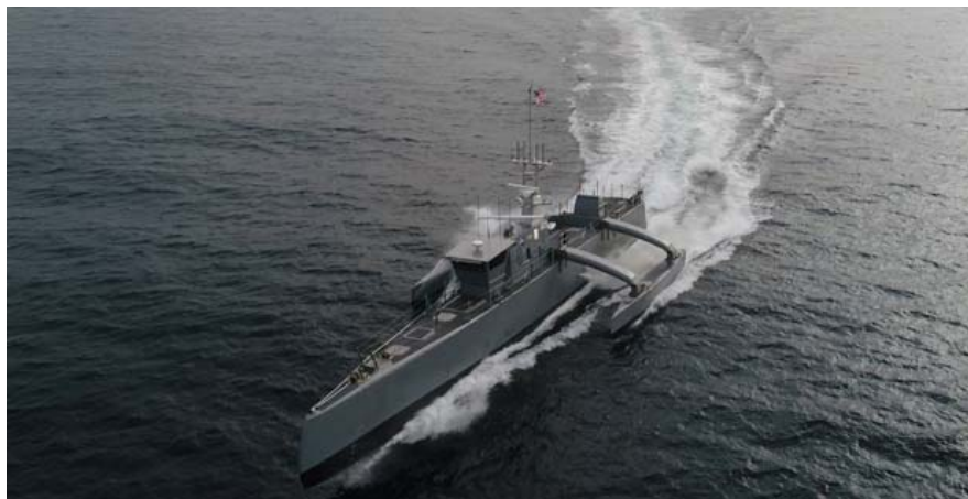
Figure 4. ACTUV "Sea Hunter" prototype developed by DARPA. Source: https://www.darpa.mil/news-events/2018-01-30a
