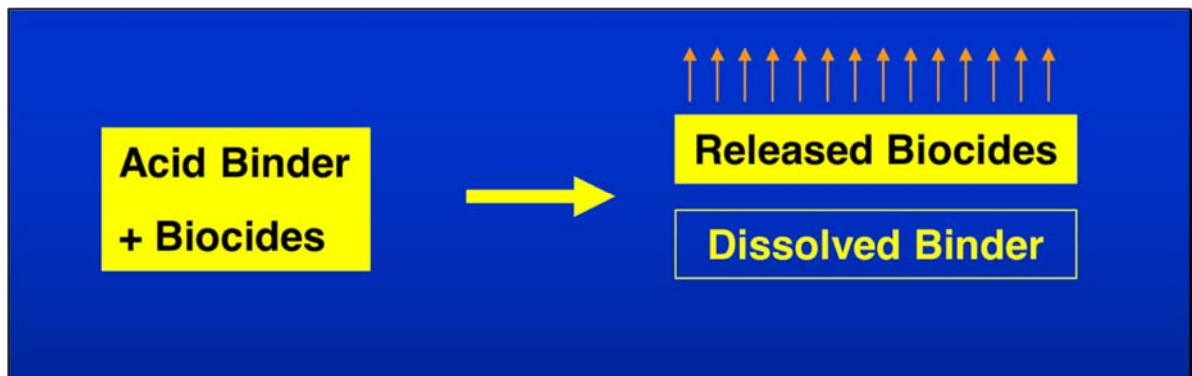
Figure 21 Chemical Process for the release of biocides.
