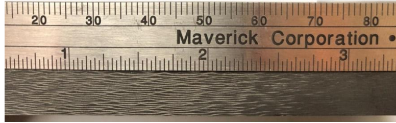
Figure 13: Cross Section of 40 Ply RM-1100 Final Composite Panel Fabricated with Experimental Cure Cycle 2, Showing Low Void Volume.
