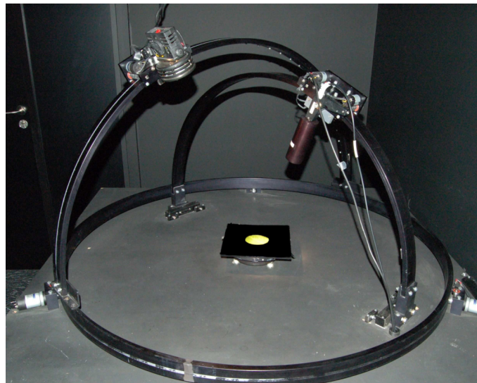
Figure 9: A custom goniometer at the Catholic University of Leuven, Netherlands. Credit: Biliouris, 2007.
