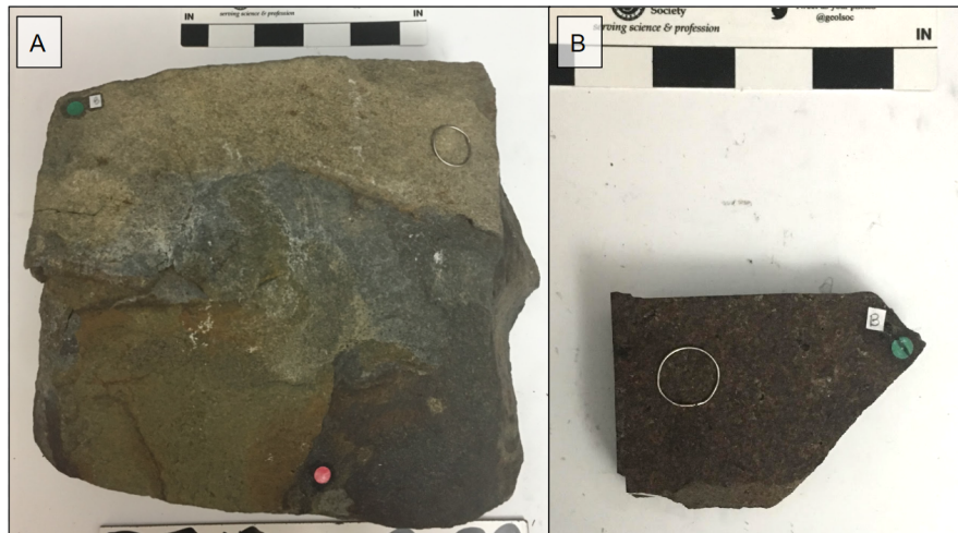
Figure 31: DF_18_003 (A) and FC_18_004 (B). These rocks represent two different types of weathering patterns seen in the sample suite, with DF_18_003 backscattering and DF_18_004 overall forward scattering. The metal ring marks the location on each rock where spectra were collected. Photo credit: Lena Gibbs.
