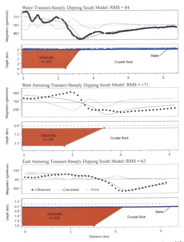
**Figure 7a.** South dipping high-angle fault models. RMS sum for this orientation is 318, the smallest misfit of the five orientations. Profiles are from south to north. "S" indicates susceptibilities, with values given in SI. Blue V's represent the locations at which measurements were taken.
