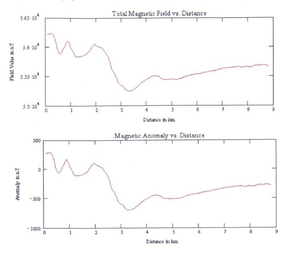
**Figure 4.** Upper graph shows raw observed field measurements for a water based transect of Cypress Island. Values are near those of the Earth's magnetic field of 55,950 nT. Lower graph is anomaly values of the same transect created by subtracting the Earth's magnetic field from the upper graph. Note minor differences in shape and positive and negative values with magnitudes less than 1000 nT. The lower graph is an anomaly profile, the data form all modeling was done with.
