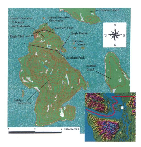
**Figure 1.** Map of Cypress Island showing relevant locations, including the two major faults and the rock units separated by the faults. The southern fault was modeled in this study. Fault traces are those mapped by Lapen (2000). Inset shows study location as white rectangle (modified from Sterner, 1995).
