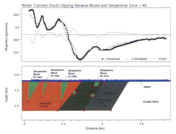
**Figure 10.** Model of water transect with high angle south dipping fault. Areas of differing amounts of serpentinization have been added to the ultramafics, and serpentine bodies have been added to the basalt (volcanic/sedimentary unit) to improve the fit of the model. South is on the left.
