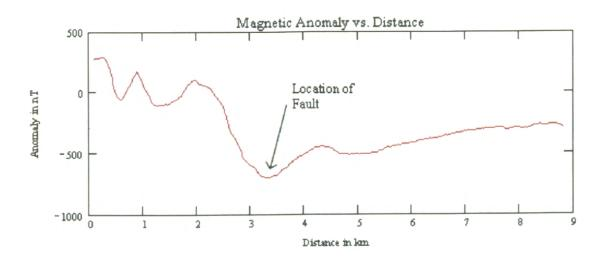
**Figure 6.** The lowest measured total field (and anomaly) value corresponds to the surface location of the fault. The location in latitude and longitude of these lowest measured values are plotted on figure 5, corresponding to the fault trace.
