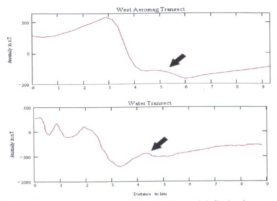
Figure 9. Anomaly increase over volcanic/sedimentary unit indicating the presence of significant amounts of magnetic material for the middle section of the island.
