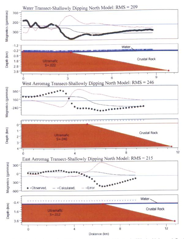
Figure 7b. North dipping low-angle fault models. RMS sum is 670, the highest misfit of the five orientations.
