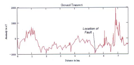
**Figure 8.** Ground transect with location of fault labeled. South is on the left. High frequency anomaly variations made this profile difficult to model, but did indicate unexpected, significant numbers of magnetic bodies in the basalt unit, north of the fault.
