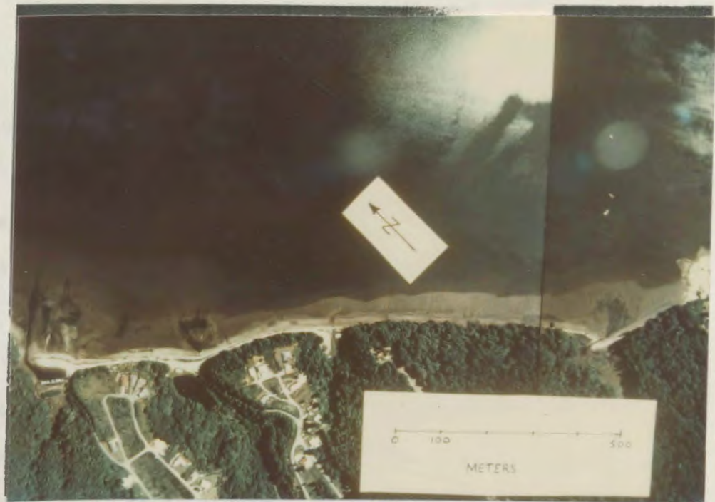
FIGURE 26a. Vertical aerial photograph showing the present coastline configuration created by the development of a small-boat marina. The marina is located within a cove that is located in the lower left corner of this photograph.
