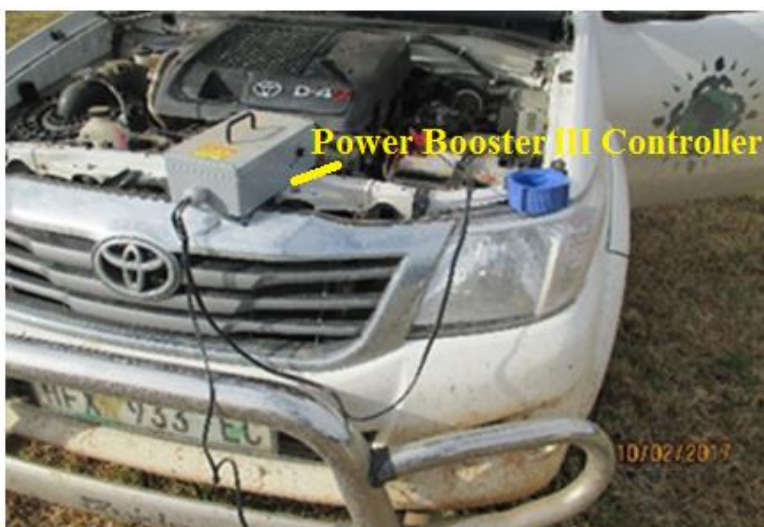
Figure 4-7: Power Booster III Controller connected to a car battery.
