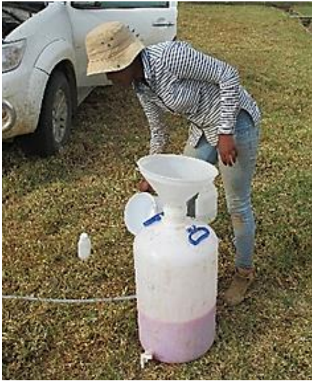
Figure 4-8: The sample water turns pink after the addition of NaOH.
