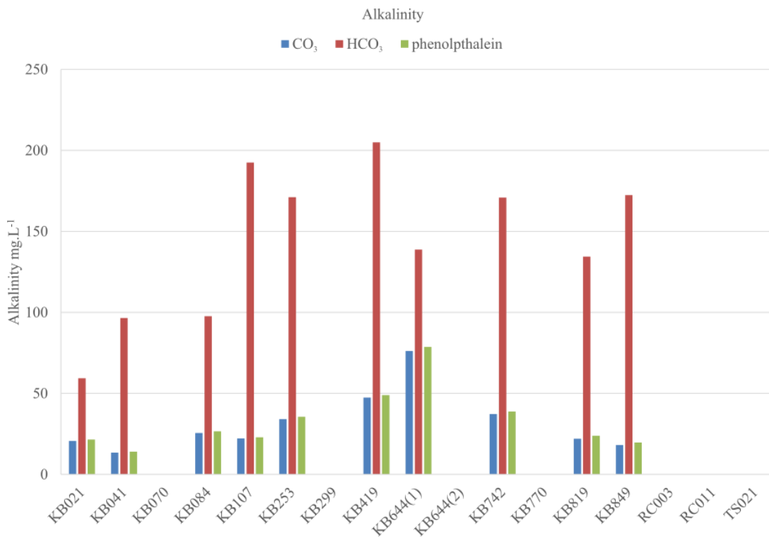
Figure 5-24: Alkalinity bar graph. Note that groundwater samples: KB070, KB299, KB644(2), KB770, RC003, RC011 and TS021 were not analysed for alkalinity.
