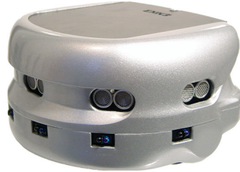
Figure 4.2: The Khepera III Robot (K-team Corporation)
