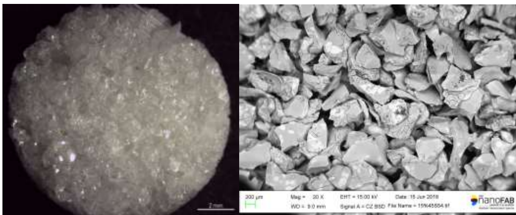
Figure 1. The liquid precursor solidifies in air to bind the 45S5 bioactive glass particles together into a rigid compact. (left) Macrophotograph of the porous composite scaffold; (right) back-scattered scanning electron micrograph of the porous composite scaffold.
