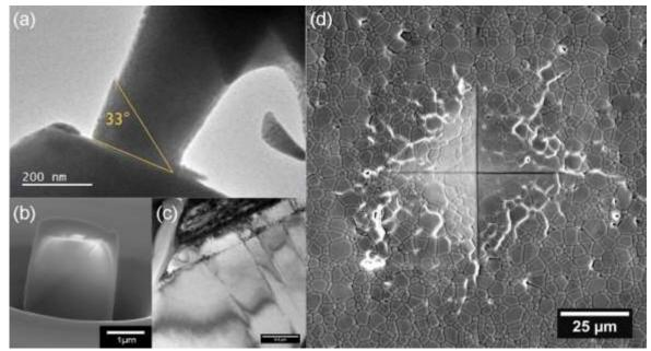
Figure 1 – An overview of the length scales probed in this study. (a) In situ single crystal nanopillar deformation as a function of crystal orientation. (b) Ex situ single crystal micropillar deformation at a lower surface to volume ratio. (c) TEM bright field imaging of the dislocation/twin structure following micropillar deformation. (d) Vickers indentation of a polycrystalline ceramic wherein twinning is observed in many but not all of the grains surrounding the indent.
