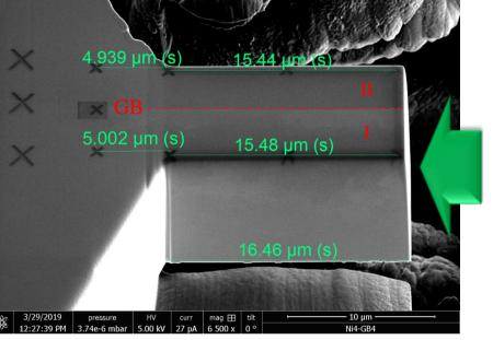
Size of the micro sample side surface: 8 µm \* 8 µm
