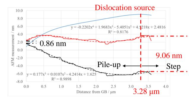
AFM measurement of slip lines, a Polynomial fit of AFM measurement and calculation weak slip transmission is observed of the number of dislocations assuming single slip
