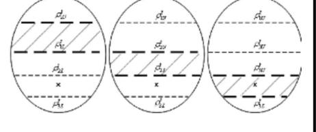
Dislocation positions in an equilibrated pile-up computed by an iterative relaxation scheme that minimizes the Peach-Koehler force on each dislocation [4]:
