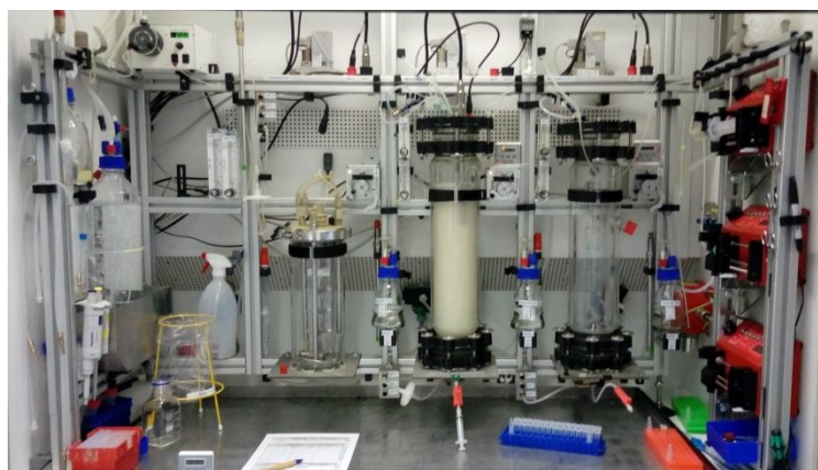
Figure 1: Experimental setup with stirred tank reactor and two 2 liter bubble column reactors for fermentative butane oxidation
