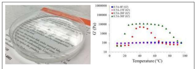
Figure 1. Left: Photograph of large, homogeneous gels. Right: Storage modulus of gels as a function of temperature for varying amounts of F127. From Quah et al., Polymer, 2018.
