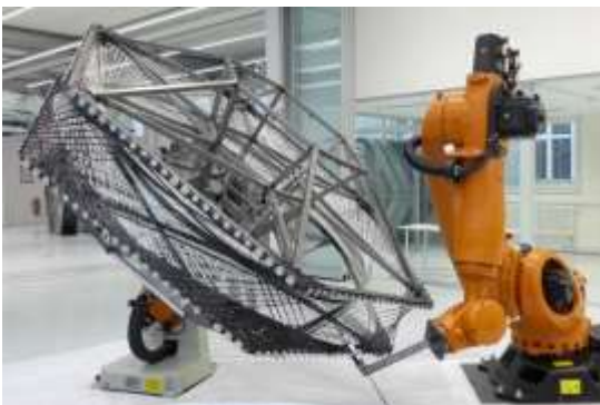
Figure 1 – Robotic filament winding of large-scale building elements
