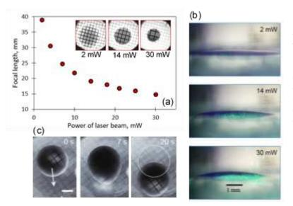
Figure 1 – (a) The droplet focal length variation vs. the laser power (images of a test-grid obtained with the droplet-lens); (b) the droplet reshaping vs. the laser power [5]; (c) The droplet motion to a new position of the laser beam [5]. Dashed circle shows the previous position of the droplet. Scale bar, 1 mm.
