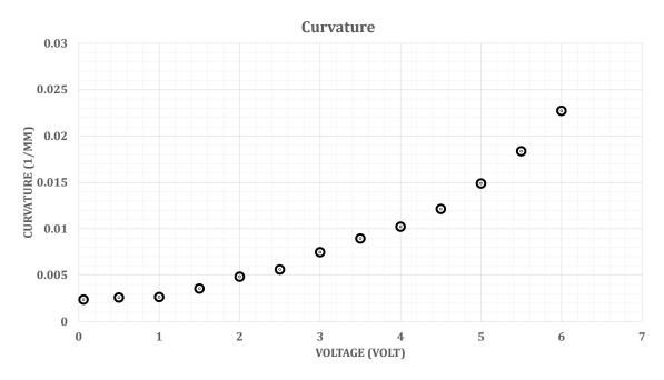
Fig. 3.15 Curvature of IPMC sample vs. applied voltage
