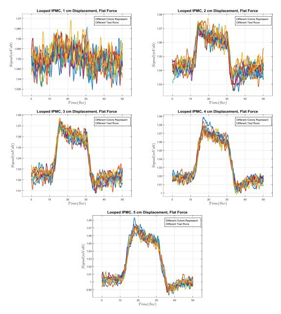
Fig. 6.12 Looped sensor stable response of Flat-tip deformation
