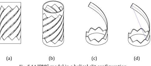
Fig. 5.14 IPMC model in a helical slit configuration
