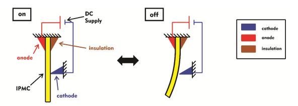
Fig. 7.1 Oscillation of IPMC with static input
