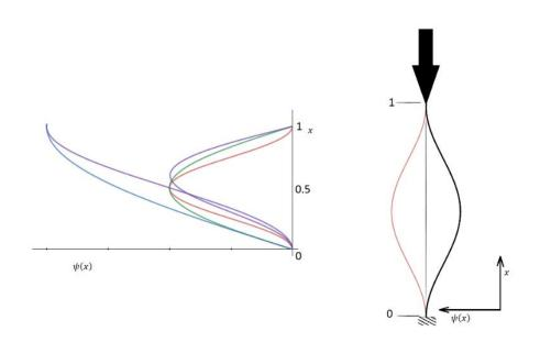
Fig. 4.6 Beam 1st Buckling mode's concepts.
