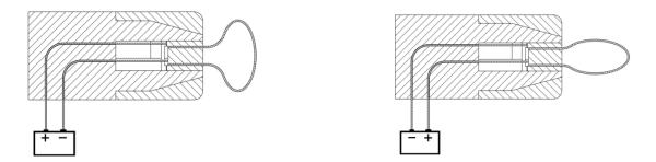
Fig. 6.1 Looped IPMCs actuator with different configurations
