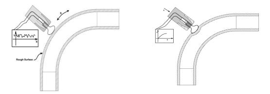
Fig. 6.2 Looped IPMCs sensor generating a haptic feedback signal
