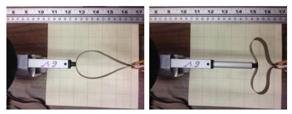
Fig. 6.6 IPMC loop sensor in haptic feedback sensing
