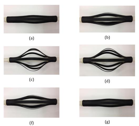
Fig. 5.10 Prototype of cylindrical IPMC actuator/sensor
