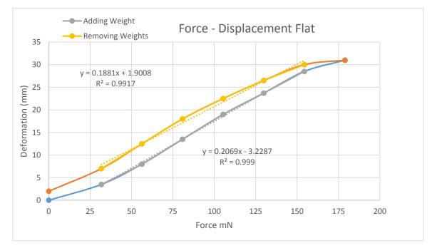
Fig. 6.27 Looped sensor configuration max. load tests
