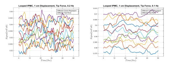
Fig. 6.8 IPMC sensing test results for 1cm displacement
