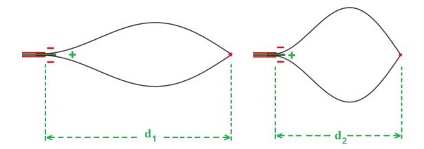
Fig. 3.18 IPMC actuator with Clamped-Hinged boundary configuration
