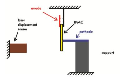
Fig. 7.2 Static Oscillatory IPMC, Test setup
