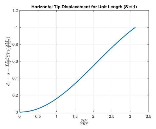
Fig. 3.7 Horizontal Tip Displacement Ratio vs. Input Voltage Ratio
