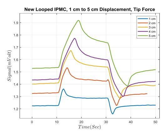
Fig. 6.35 Smother test results of the new IPMC haptic feedback sensor
