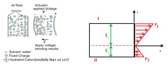
Fig. 3.2 Essential mechanism of actuation in IPMC
