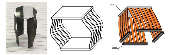
Fig. 5.6 Circular and rectangular assembly of IPMC sensor/Actuators
