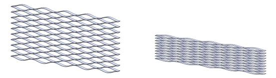
Fig. 7.29 2D metamaterials made with an assembly of pairs of IPMC strips
