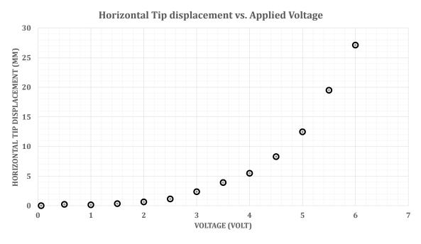
Fig. 3.14 Horizontal Tip displacement of IPMC sample vs. applied voltage
