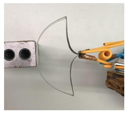
Fig. 6.37 Alternate form of New version of an IPMC haptic feedback sensor
