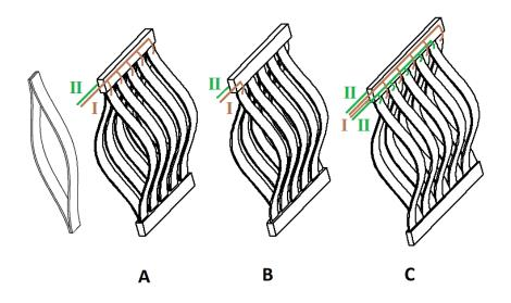
Fig. 5.5 Example of attaching multiple sensors
