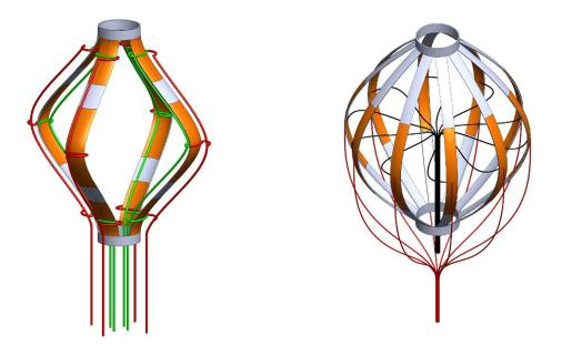
Fig. 5.15 Demonstration of wiring for slit cylindrical IPMC actuator/sensor
