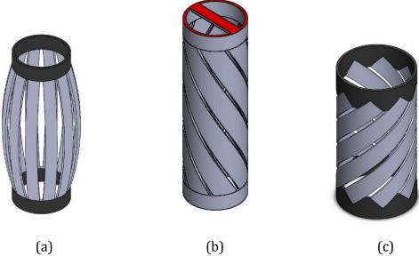
Fig. 5.11 Cylindrical, and Helical form of IPMC actuator/sensor
