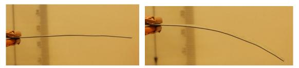
Fig. 3.12 IPMC sample in actuation with voltage variation
