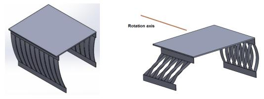
Fig. 7.20 the rotatory table made by IPMC actuator
