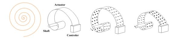
Fig. 7.28 Using IPMC as a shaft Controller to rotate a shaft
