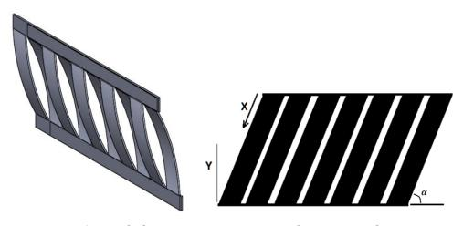
Fig. 5.9 Angled arrangement concept of IPMCs membrane
