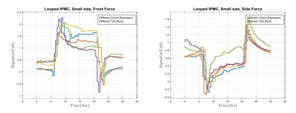
Fig. 6.30 Results of IPMC haptic feedback sensor for surgical end-effector
