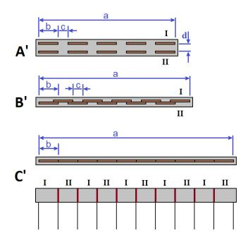
Fig. 5.3 Boundary connections of IPMC assembly
