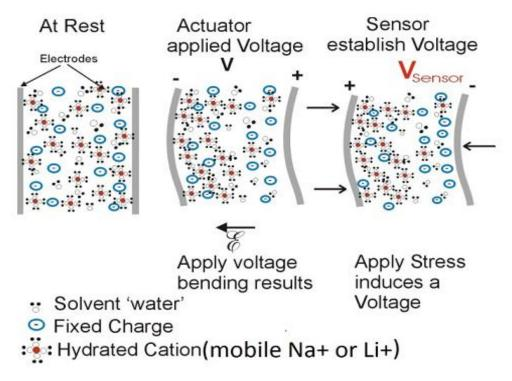
Fig. 2.1 The essential mechanism of actuation and sensing in IPMC
