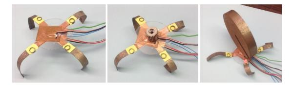
Fig. 7.15 Stewart platform robot with IPMC legs being able to carry weight
