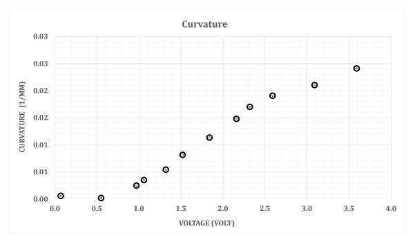
Fig. 3.11 Curvature of IPMC sample vs. applied voltage
