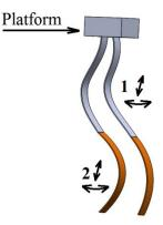
Fig. 7.23 Walking biped with tow strip of IPMCs for each leg
