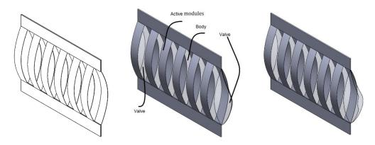
Fig. 7.18 Assembly of the linear actuators with higher capacity
