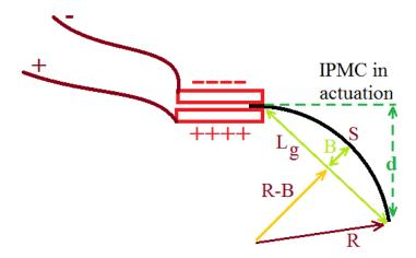
Fig. 3.5 Dimensional representing IPMC in actuation
