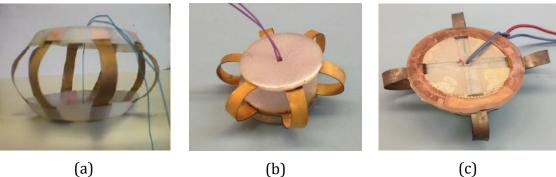
Fig. 7.13 Tubular silted IPMC linear actuator/sensor, device
