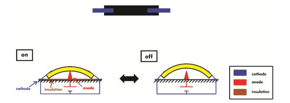
Fig. 7.5 Oscillatory IPMC in a dome shape configuration
