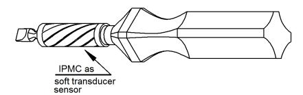
Fig. 7.25 Application concept of slit cylindrical helical IPMC
