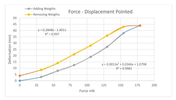
Fig. 6.26 Looped sensor configuration max. load tests
