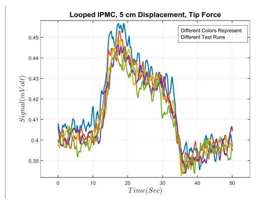
Fig. 6.7 IPMC sensing experimental results for a 5cm displacement
