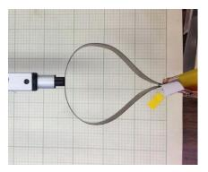
Fig. 6.3 IPMC sample original form and the looped form
