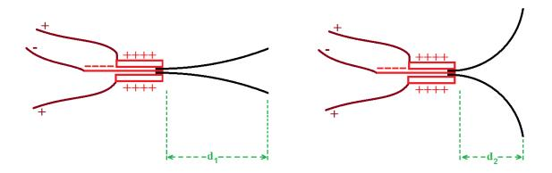
Fig. 3.16 IPMC actuator with Clamped-Free boundary configuration
