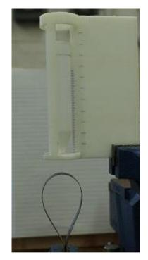
Fig. 6.24 test setup for Looped sensor for the force-displacement
