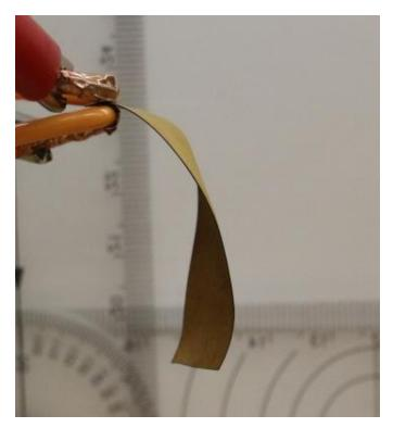
Fig. 3.1 Bending and Twisting Deformation of an IPMC sample
