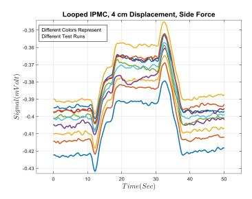
Fig. 6.36 signal of side test on haptic feedback of a loop sensor
