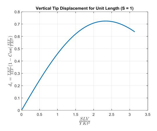
Fig. 3.6 Vertical Tip Displacement Ratio vs. Input Voltage Ratio
