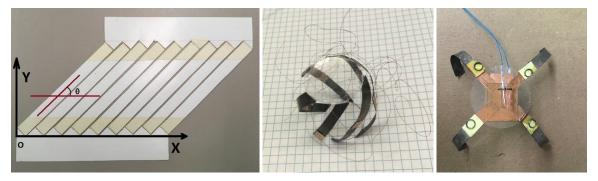
Fig. 5.8 Prototype models for assembly of IPMC sensor/actuator
