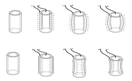
Fig. 7.10 Expansion and contraction of cylindrical tubular IPMC
