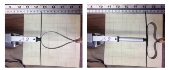
Fig. 6.11 Looped IPMC being pushed by a linear actuator on a flat surface
