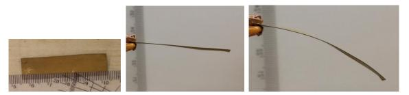
Fig. 3.8 IPMC sample in actuation with voltage 0.55 Volts and 2.16 Volts
