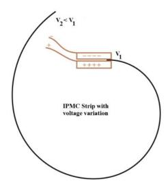
Fig. 3.4 Graphical representation of a spiral IPMC sensor/actuator
