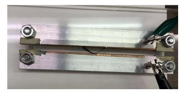
Fig. 7.7 Test setup for Oscillatory IPMC in a straight contact channel
