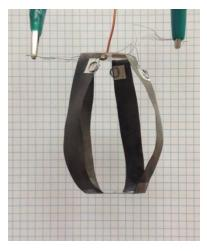
Fig. 5.7 Actuation of a slit cylindrical IPMC actuator
