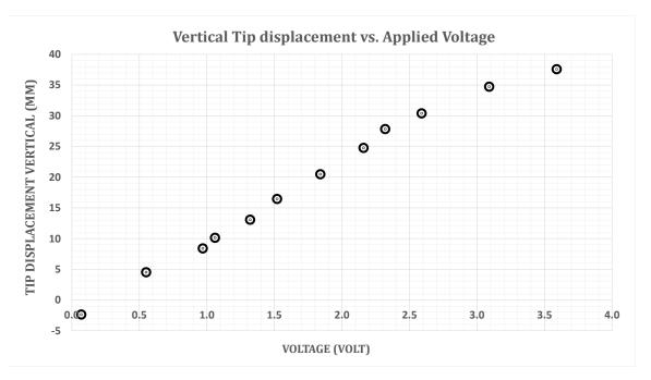
Fig. 3.9 Vertical Tip displacement of IPMC sample vs. applied voltage
