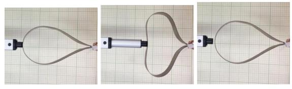
The initial gap betweenHolding for 1 min at 3cmFinal Gap for 3cmthe actuator and the loopDisplacementDisplacementFig. 6.10 Looped concernt temporary deformationfor 3cmdeformation
