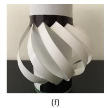
Fig. 5.12 Deformations and twisting of IPMC as helical actuator/sensor.
