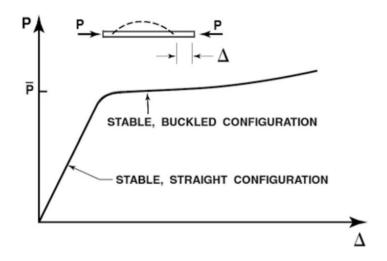
Fig. 4.5 IPMC axial load variation under axial compression load
