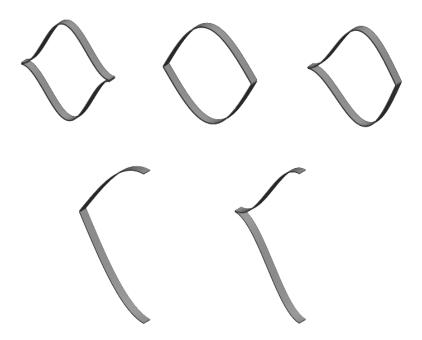
Fig. 5.1 Basic configurations of pairs of IPMC sensors
