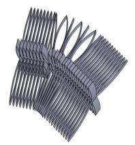
Fig. 7.27 3D curve controller made by pairs assemblies of IPMC strips
