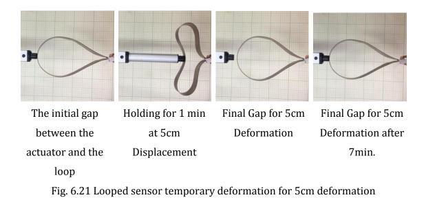
6.3.2 Looped IPMC Free End vs. Attached End
