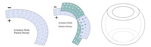
Fig. 7.9 Scheme of distribution of cations for IPMC in actuation mode
