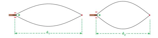
Fig. 3.19 IPMC actuator with Hinged-Hinged boundary configuration
