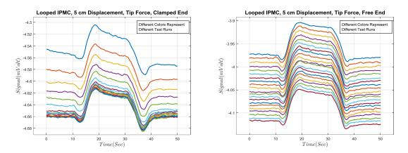
Fig. 6.22 Looped sensor generated signal for 5cm deformation
