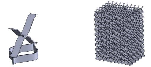
Fig. 7.30 3D metamaterial element made with pairs of IPMC strips
