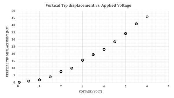
Fig. 3.13 Vertical Tip displacement of IPMC sample vs. applied voltage
