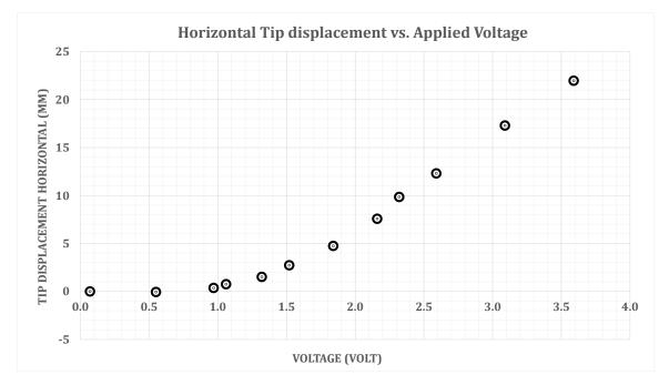
Fig. 3.10 Horizontal Tip displacement of IPMC sample vs. applied voltage
