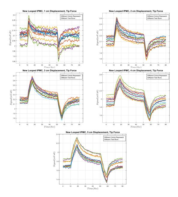
Fig. 6.33 New Looped sensor stable response of Point tip deformation
