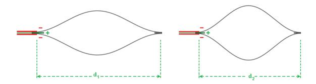
Fig. 3.17 IPMC actuator with Clamped-Clamped boundary configuration
