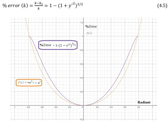
Fig. 4.7 Variation of error for simplified curvature equation
