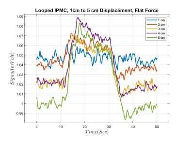
Fig. 6.13 Looped IPMC response voltage signal to Flat point force
