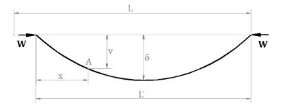
Fig. 4.13 An elastic beam material under axial load-deformation
