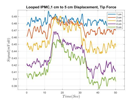
Fig. 6.9 Looped IPMC response voltage signal to tip point force
