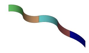
Fig. 7.24 Attachment of several IPMC strips to form a snake-like-robot
