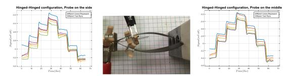
Fig. 4.10 Sensing signal of IPMC sample with Hinged-Hinged configuration
