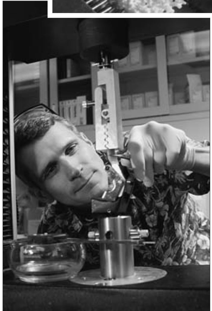
UMaine engineer Darrell Donahue will use specialized equipment to measure the strength and efficacy of foam metal implants.
