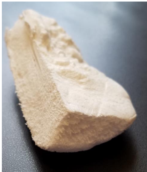
Figure 2.5: Ridged foam CNF vial lyophilization
