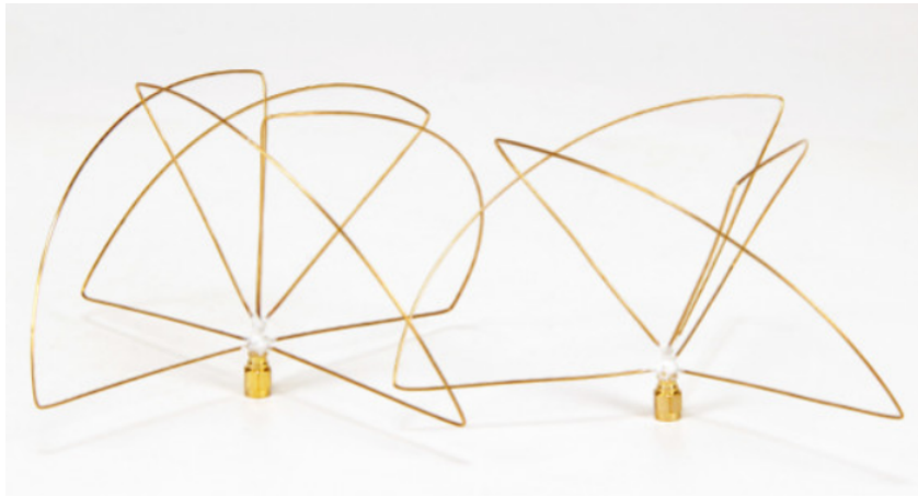
Figure 3.30: Design 3 - Payload Antenna: Cloverleaf Antenna 3 and 4 leaves.
