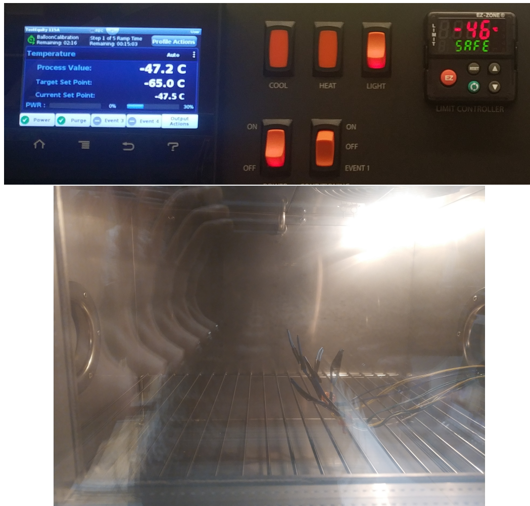
Figure D.4: Temperature chamber calibration controls and thermistors being calibrated.
