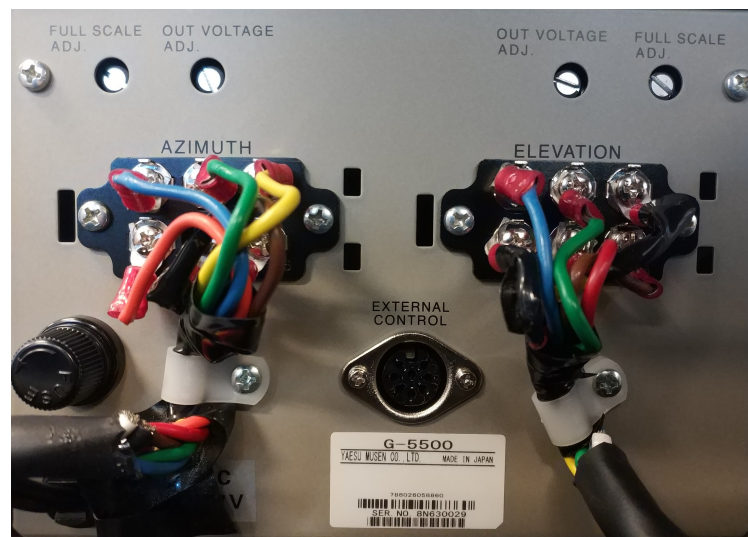
Figure 3.6: Rotor Controller - Box Calibration Adjustments
