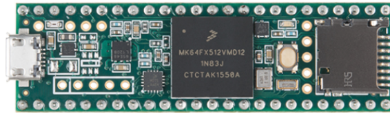
Figure 3.29: Design 3 - Payload Controller: Teensy 3.5 ARM Cortex M4 MCU.
