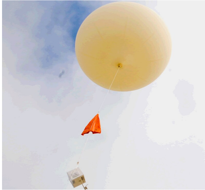
Figure 1.1: Weather balloon, top; parachute, middle, radiosonde instrument, bottom (National Weather Service).
