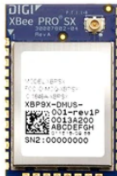
Figure 3.24: Payload Surface Mount Module with u.fl antenna connector.
