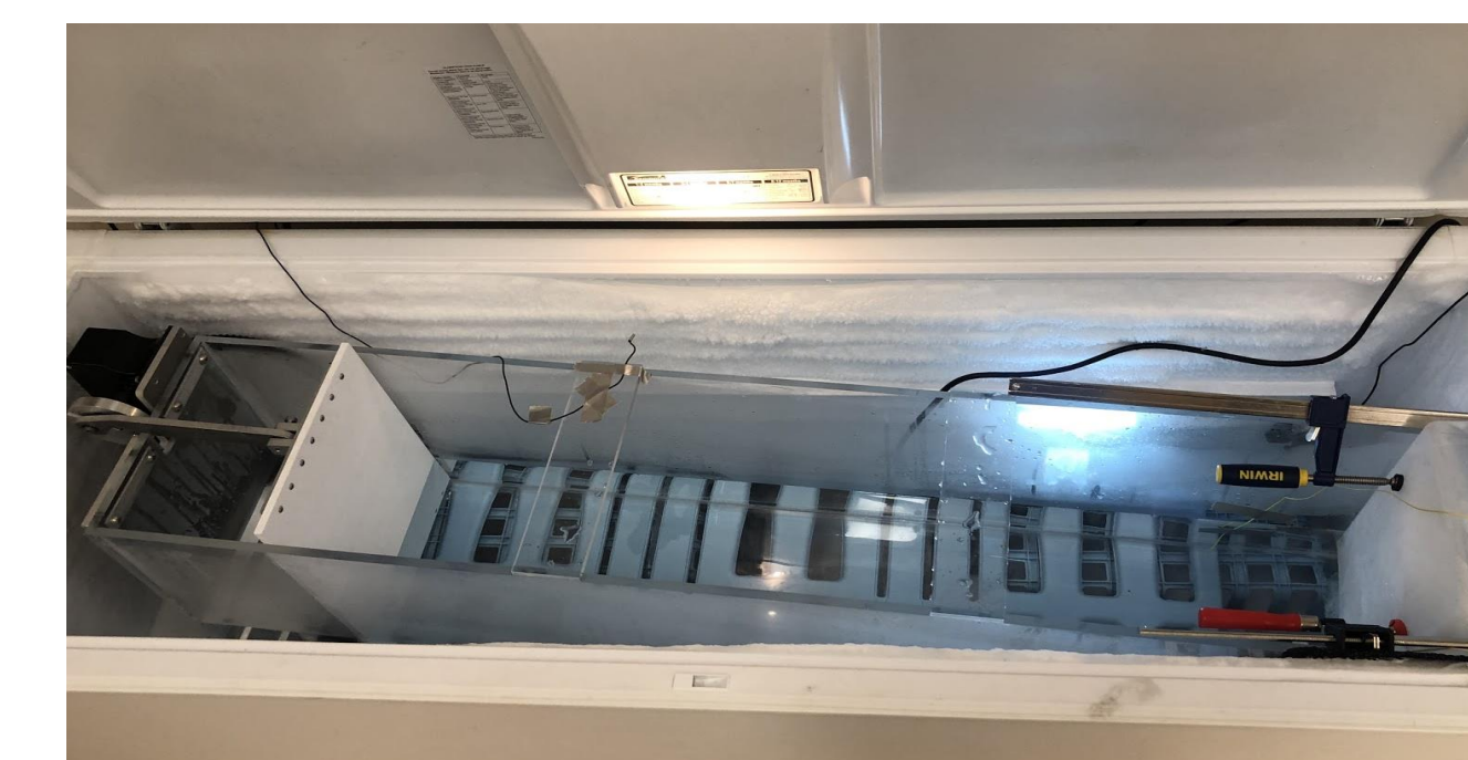
Figure 5: Temperature-controlled experiment setup, in which wave tank was placed into chest freezer.
