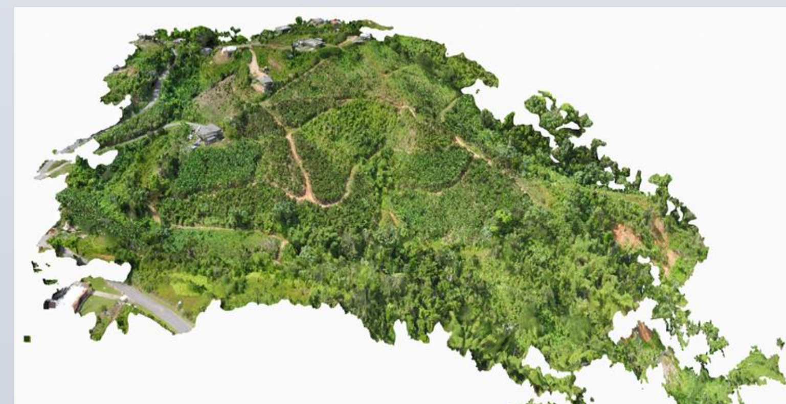
Figure 4. 3D digital surface model created in Pix4D.
