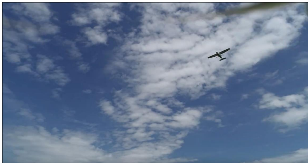
Figure 9. Excerpts from sUAS video taken prior to aircraft overflight of sUAS with aircraft highlighted in red: (Top) 30 seconds prior; (Middle) 10 seconds prior; (Bottom) 2 seconds prior. Long-range identification was nearly impossible without relying on spotting the aircraft's wig-wag LED landing lights. Full video available at: https://commons.erau.edu/ijaaa/vol6/iss5/12/
