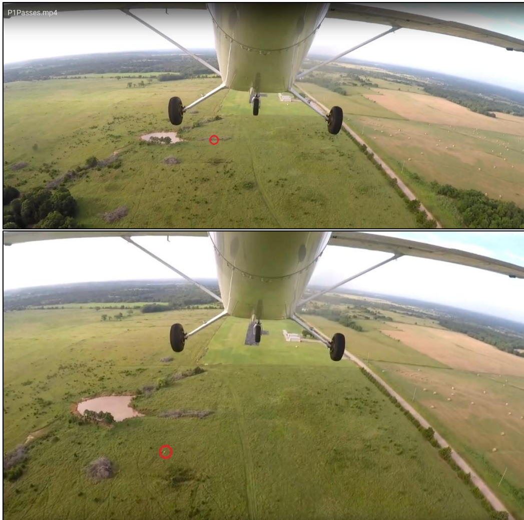
Figure 10. Excerpts from externally-mounted video camera taken during Participant 1, Intercept 2. Note the relatively small size makes the sUAS extremely difficult to detect. The participant did not detect the sUAS during this pass. Full video available at: https://commons.erau.edu/ijaaa/vol6/iss5/12/
