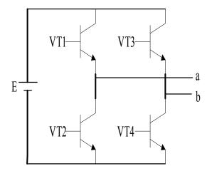
Figure 2-3 H-bridge basic power unit structure
