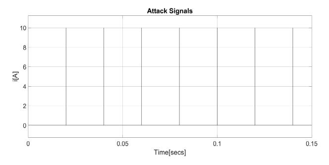
Figure 2-12 Pulse attack signals
