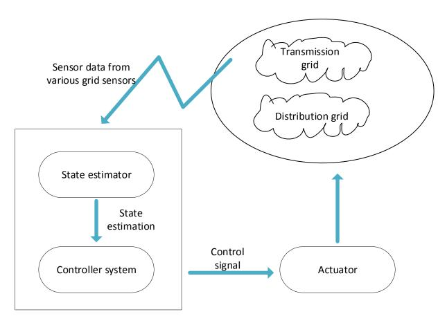
Figure 3-1 Block diagram of smart grid system
