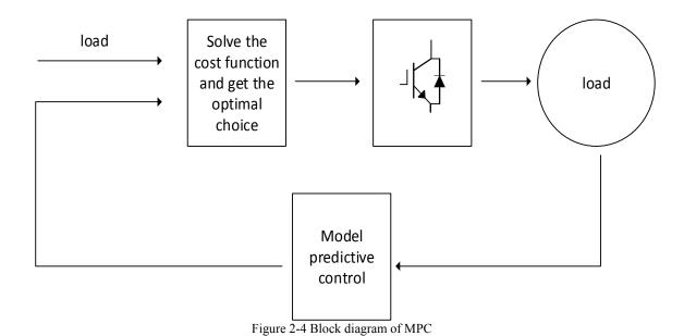
The principal idea of model prediction current control algorithm makes predictions of load current generated by every feasible voltage vector at next moment of the inverter, and choose the optimal voltage vector that has minimum value acting on inverter at following moment for load current tracking. The mechanism of MPC is presented in Figure 2-4.
