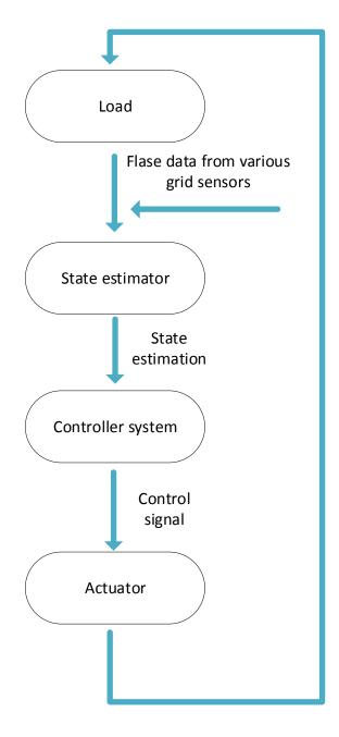
Figure 3-8 Block diagram of control steps
