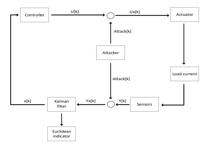
Figure 3-7 Block diagram of FDIA on forward ad feedback
