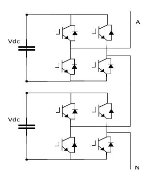
Figure 2-1 The symmetrical Cascaded H-Bridge multilevel inverter Topology
