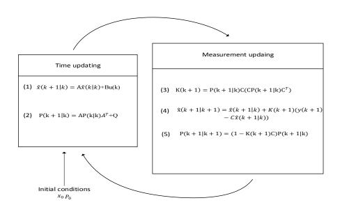
Figure 3-2 Block diagram of Kalman Filter
