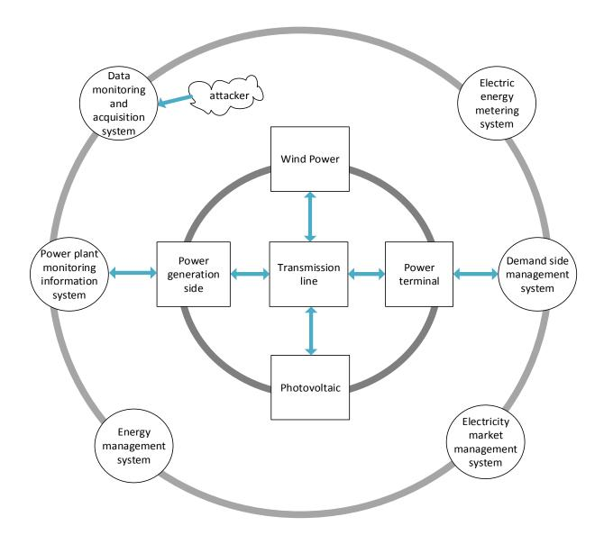
Figure 1-4 The framework of cyber physical power system
