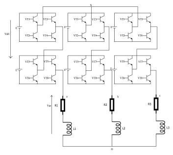
Figure 2-2 Three-phase five-level H-bridge inverter topology
