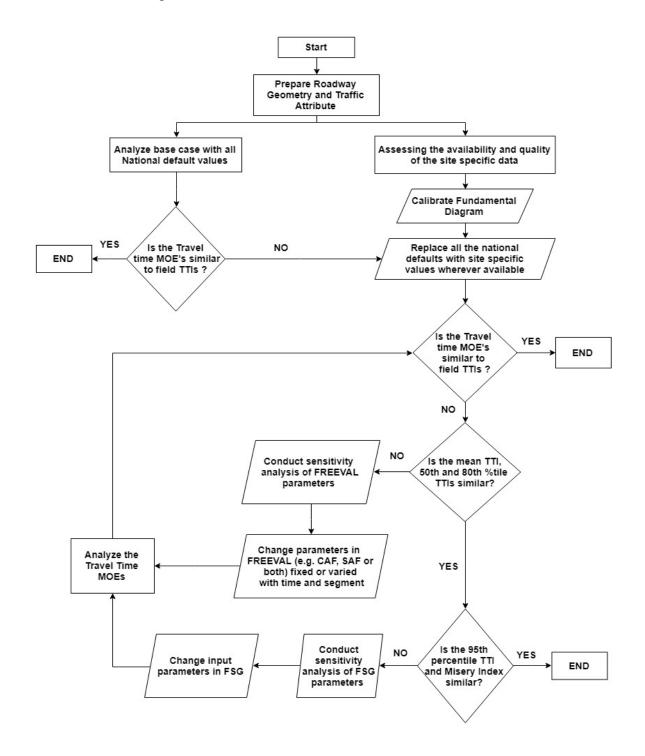
**Figure 5-1:Calibration Procedure**
