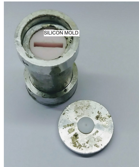
(b) Mold for Shaping Particle-Epoxy Slurry into Rectangular Slab
