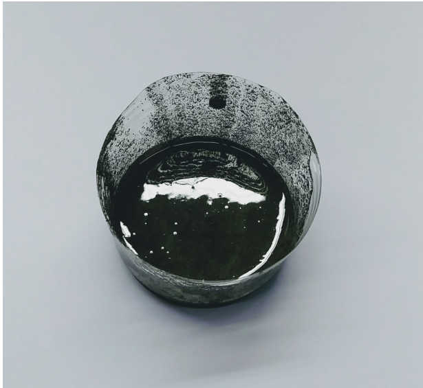
(a) Terfenol-D/Epoxy Composite
