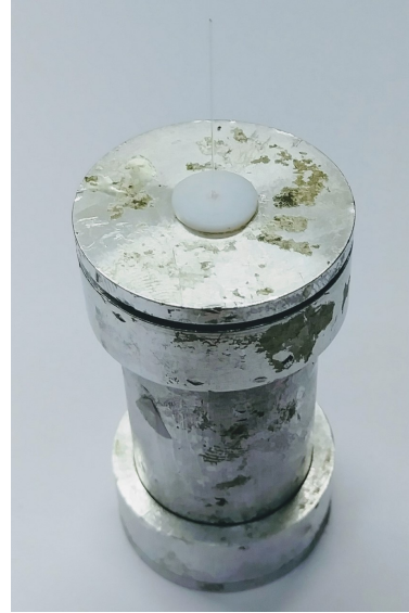
(b) Composite with FBG inside the Mold
