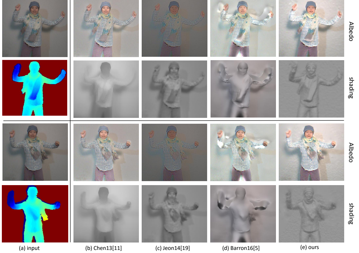
Figure 4.3: Results on sampled images from hand waving stream. (a) Input color image and depth map. (b-e) Albedo and Shading images estimated by three recent approaches for intrinsic decomposition and by our approach.
