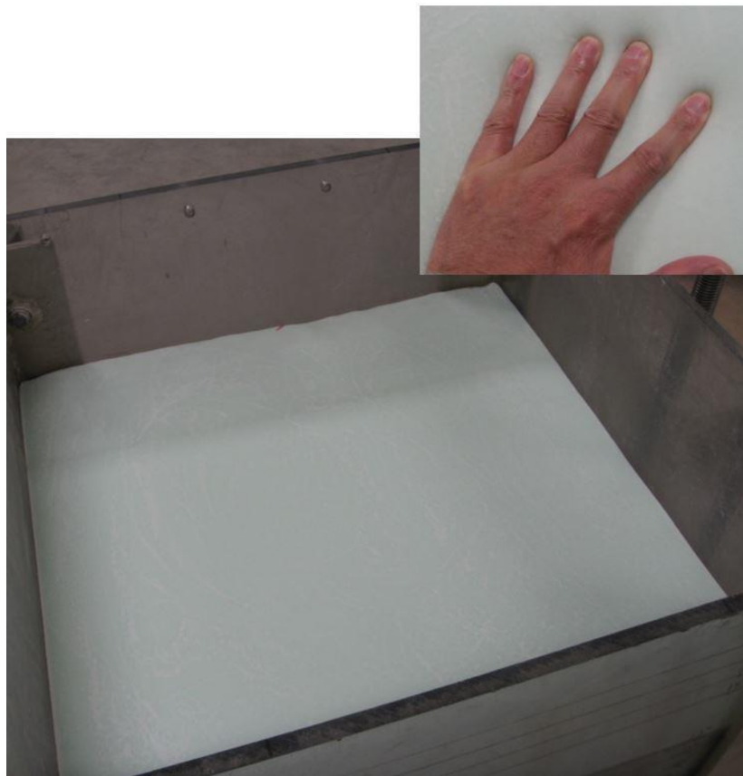
Figure 13. Pudgee – used to simulate weak soil.
