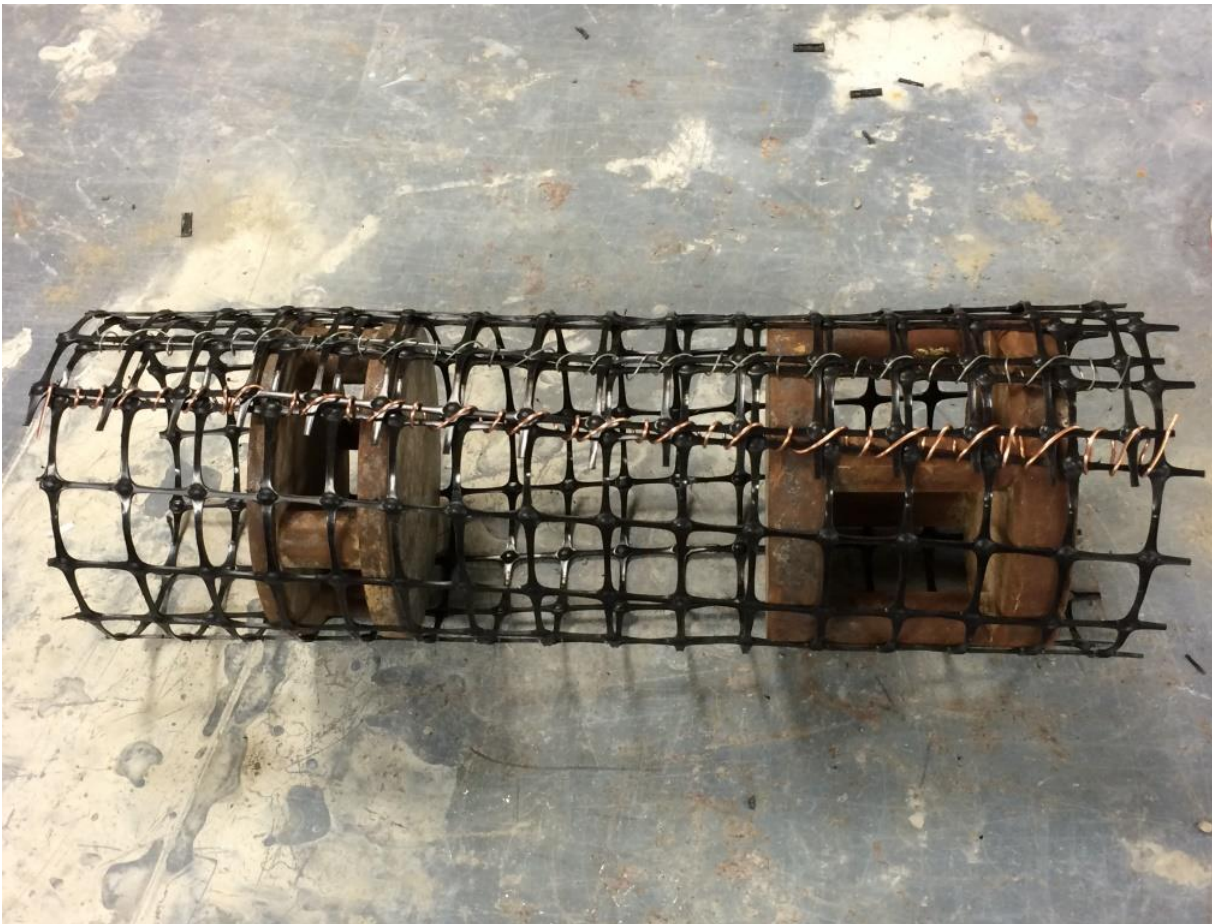
Figure 1. Geogrid wrapped on 5\text{-}7/8 in. cylinder with two rows of geogrid connections by using wires to make 5\text{-}7/8 in. inner diameter and 15 in. long cylinder.
