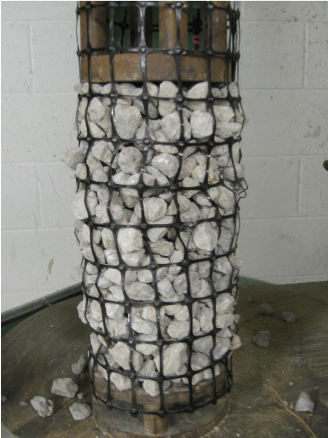
Figure 5. Cylindrical geogrid filled with crushed stone sample failure.
