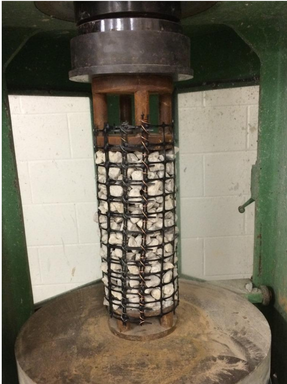
Figure 3. Place geogrid caged crushed-stone cylinder with a \phi 5\text{-}7/8 in. metal cylinder above crushed stone top on compression test machine.
