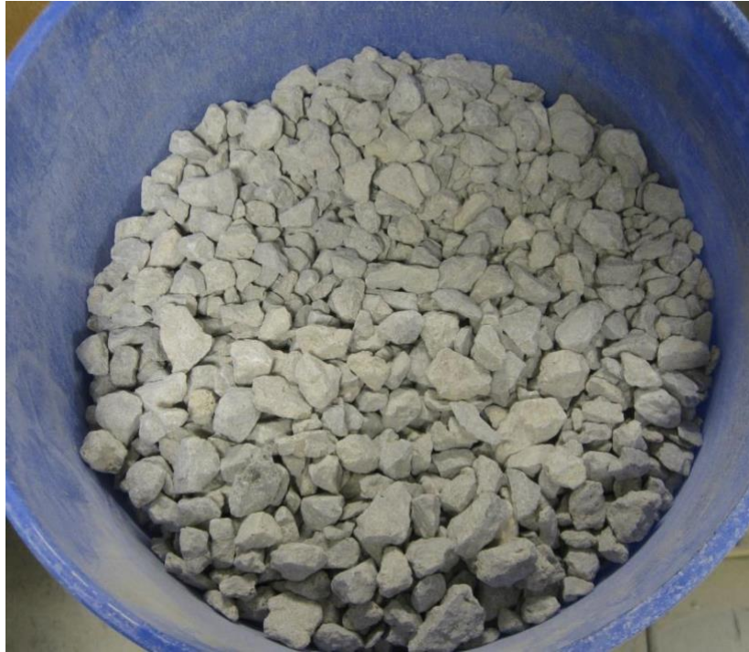
Figure 14. Crushed stone – used to interact with geogrid.
