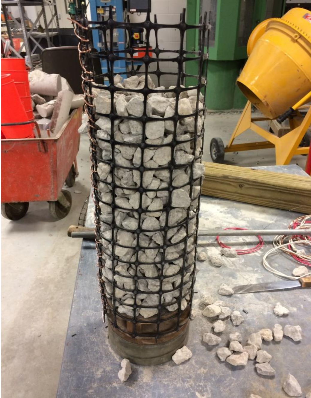
Figure 2. Fill the crushed stone in the geogrid cage to form a \phi 5-7/8 in. by 12 in. geogrid caged crushed stone cylinder.
