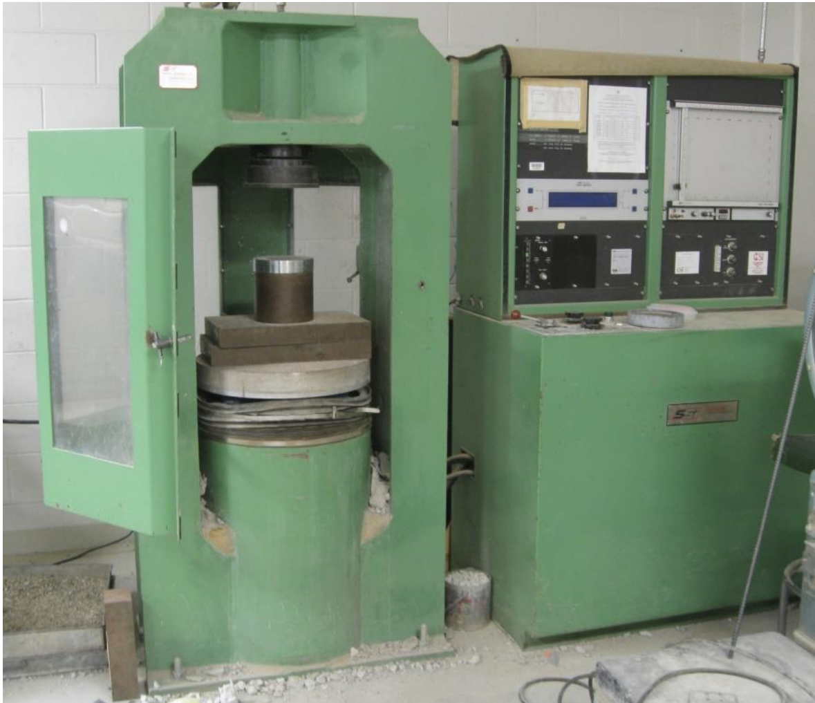
Figure 4. A compression test machine with maximum load 400 kips.
