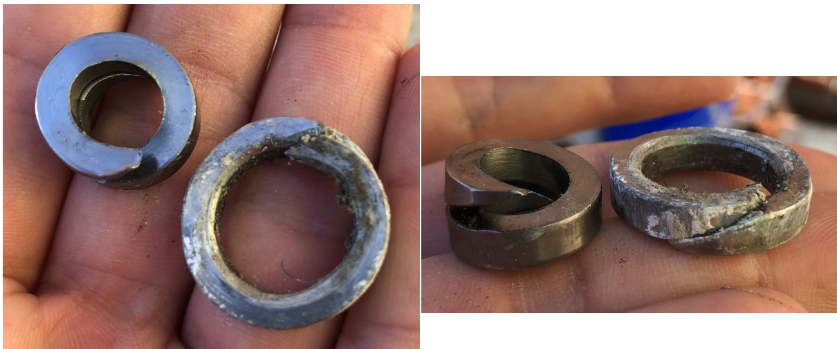
Figure 9 The expandable insert expanded before and after. The left insert in both pictures is the shape before expansion; the right one in both pictures is the shape after expansion.
