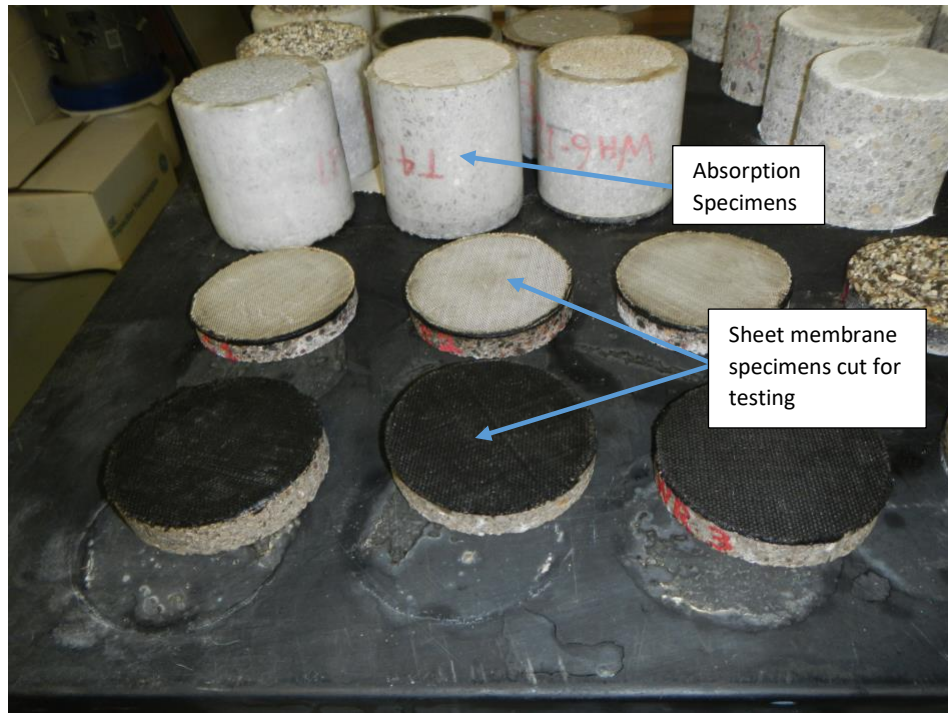
Figure 3 Specimens after cutting to length
