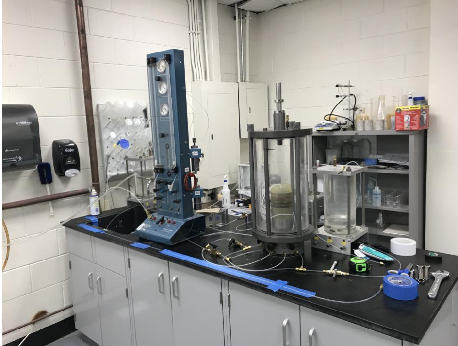
Figure 5 Permeameter with vacuum capability
