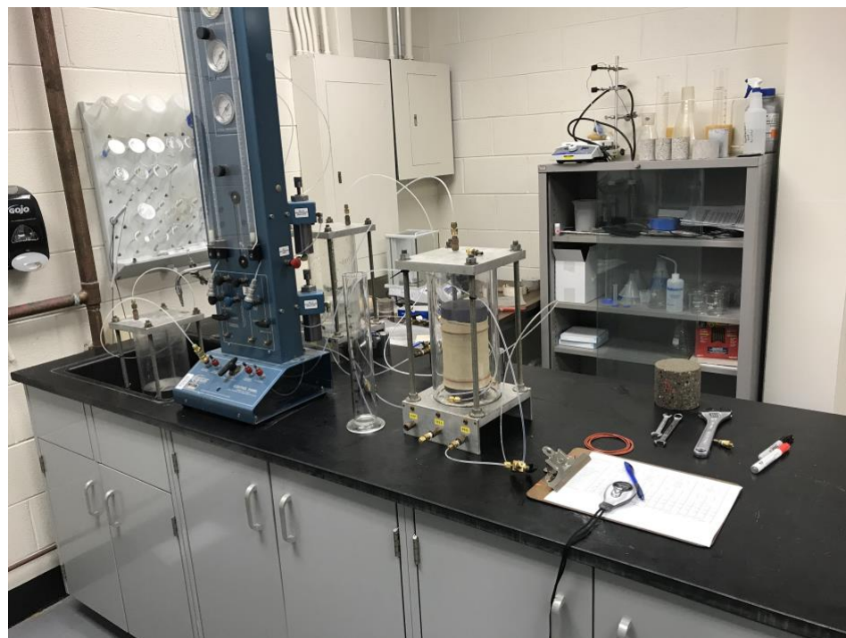
Figure 4 Small Permeameter without vacuum
