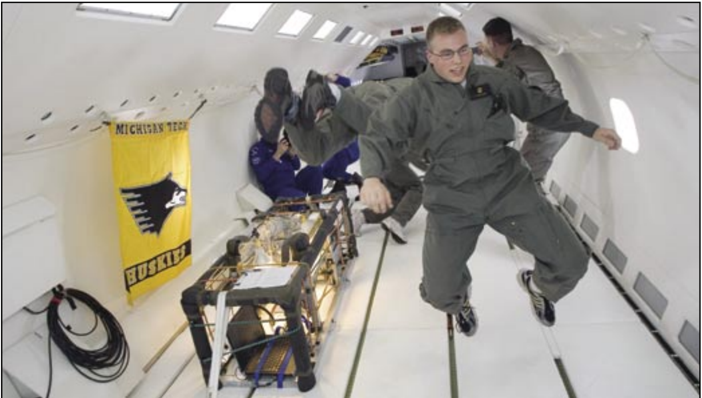
Mechanical Engineering student and Aerospace Enterprise team member EJ Meyer experiences reduced gravity while running an experiment aboard a NASA zero gravity simulator aircraft. The experiment investigates using electrostatic fields to remove lunar dust from solar cells.
