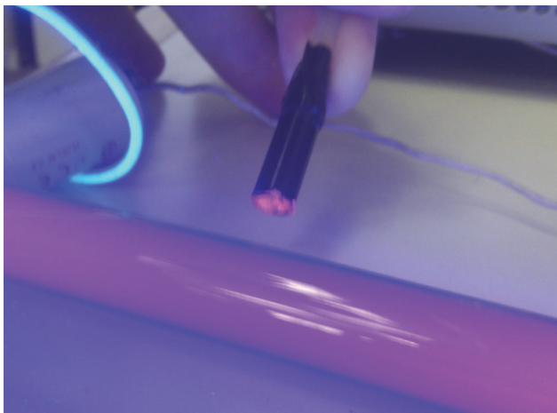
Fig. 4. End-type sensor with powder from mercury lamp.
