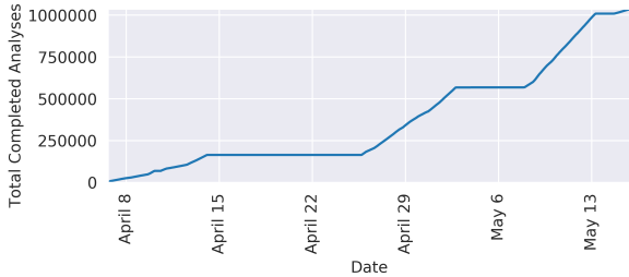
Fig. 2. The progression of app analyses during our Play Store sweep, which ran for 512 hours at an average rate of 2,023 apps/hour.
