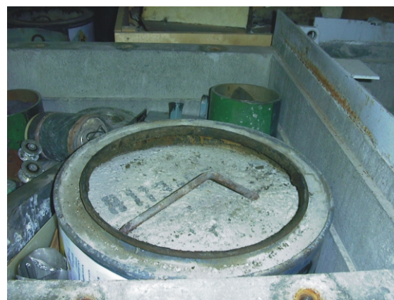
Figure 6. Cementation of radioactive waste in concrete container
