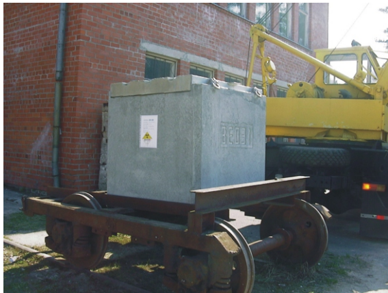
Figure 7. Radioactive waste in concrete container is ready for transportation
