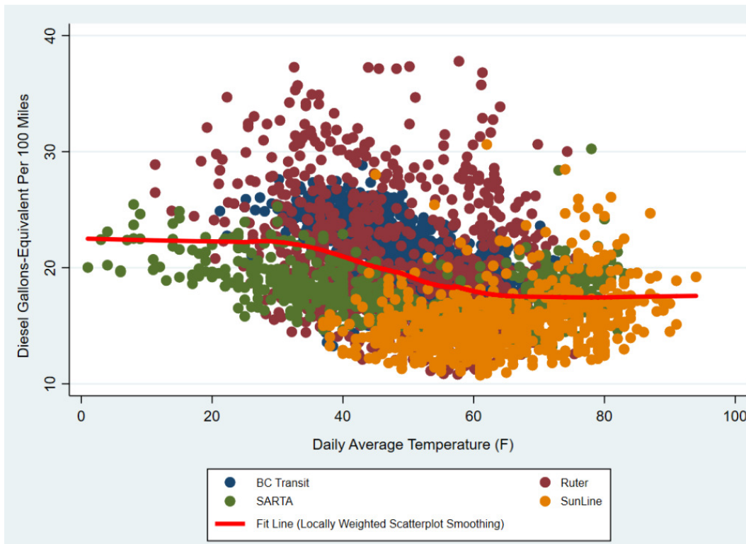
Figure 2. Diesel Gallons-Equivalent Per 100 Miles Fuel Economy for FCEBs
