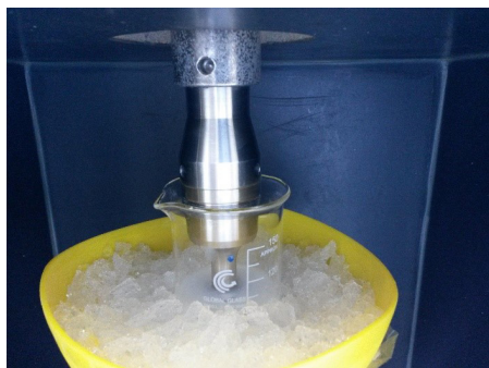
FIGURE 1 Beaker immerse in ice for NCC dispersion using a Branson digital sonifier.
