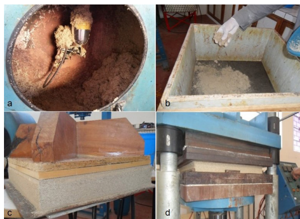
FIGURE 2 Particleboard production. Adhesive dispersion (a), particle mattress formation (b), mattress after pre pressing (c) and hot pressing (d).
