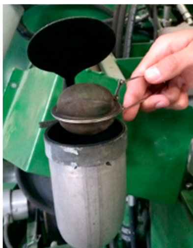
Figure 1. The exhaust pipe and the filter with weed seeds.
