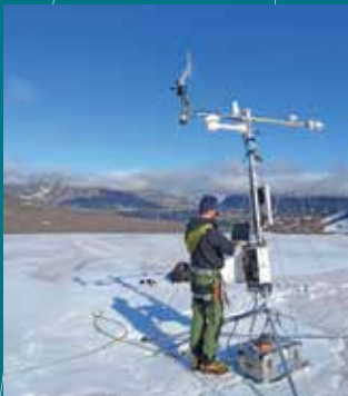
The LYN-1 automatic weather station during maintenance, on the tongue of Chamberlin glacier. Photo: Laura H. Rasmussen, KU.
