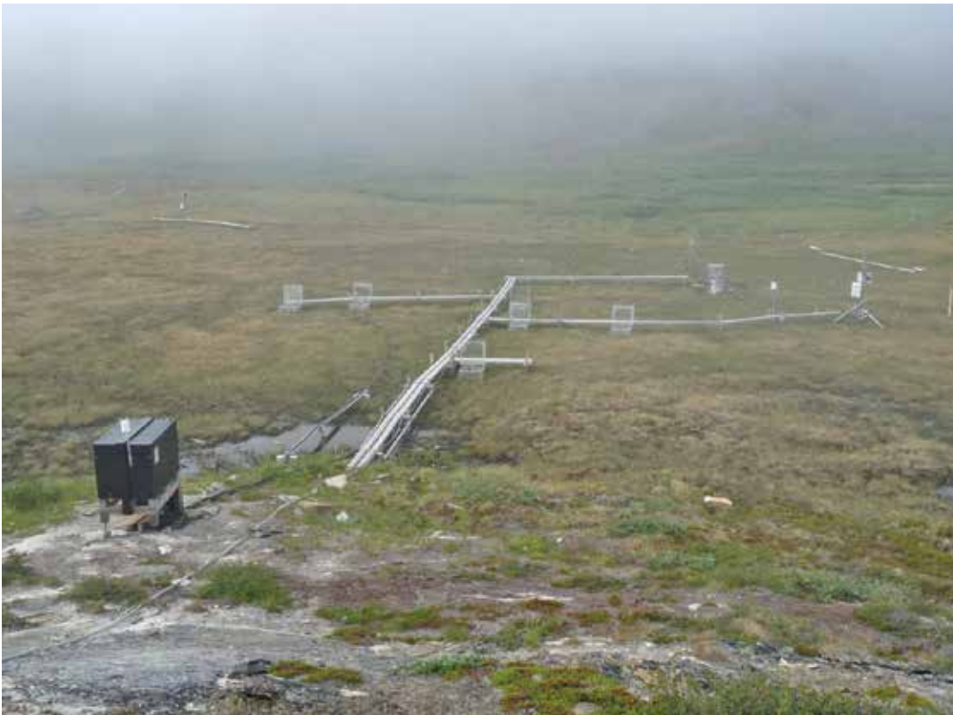
The flux measurements and energy exchange stations (here from Kobbefjord) with surface temperature sensors and radiation pyranometers (rightmost mast) are central for the correction of remotely sensed skin temperatures, especially in cloudy conditions (Photo: Antti Lauri).
