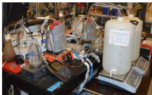
Figure 1. The two FO-AnMBRs reactors' setup
